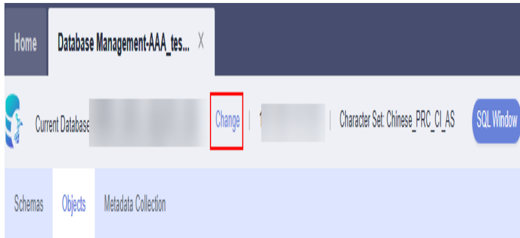
Figure 4-62 Switching to the database where you want to view details of a stored procedure
