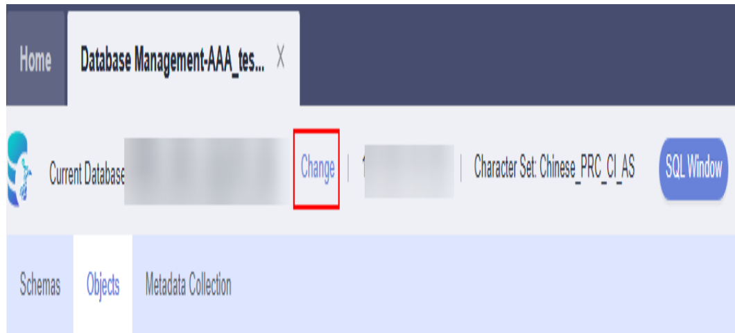
Figure 4-56 Switching to the database where you want to alter or execute a stored procedure
